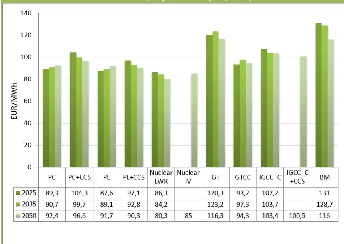
Fig. 4.11. Averaged unit energy generation costs for sources envisioned for commissioning in 2025, 2035 and 2050, resp. – at CF 0.8 [EUR/MWh].
