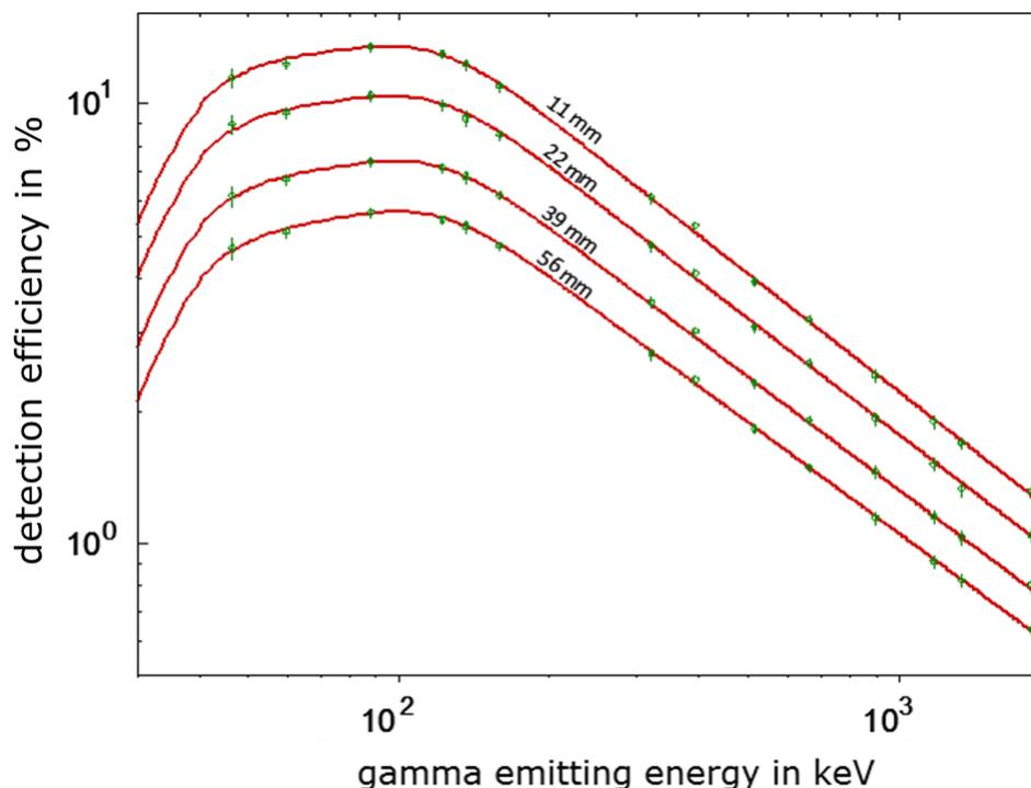
**Fig. 2:** Determined detection efficiency in % and fitted calibration curves for different filling heights between 11 mm and 56 mm, ordered from top to bottom; the calibration was carried out on an n-type detector with aluminum endcap.
