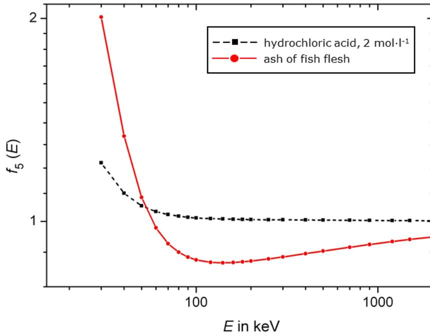
**Fig. 3:** Calculated self-attenuation correction factors as function of the gamma-ray energy after calibration using hydrochloric acid ( $2 \text{ mol}\cdot\text{l}^{-1}$ ) and in ash from fish flesh; the filling-height are 40 mm, the density of the ash is  $0,47 \text{ g}\cdot\text{cm}^{-3}$  and that of hydrochloric acid  $1,03 \text{ g}\cdot\text{cm}^{-3}$ .
