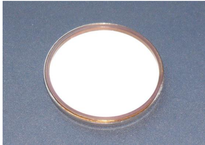
Fig. 3: Filter cake fixed in the measurement tray by means of a retainer ring.
