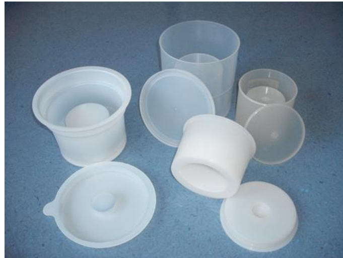
Fig. 2: Examples of common Marinelli beakers
