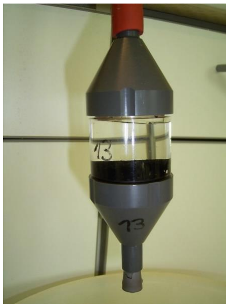
Fig. 5: KCFC filled ion exchange column
