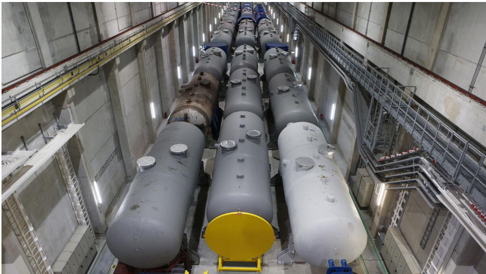
Figure D-7: Decay storage of large components (steam generators) at the Storage Facility North (Copyright: EWN)
