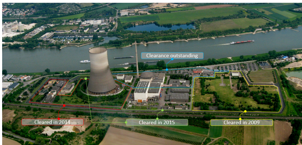
Figure D-21: Division of the Mülheim-Kärlich nuclear power plant site into four sections for clearance (Copyright RWE AG)
