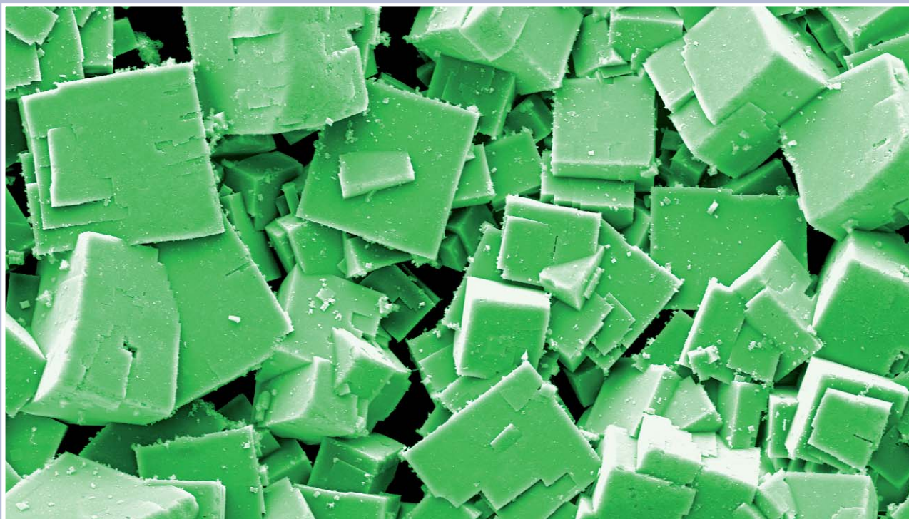
Figure 25: Nano cubes for hydrogen storage
