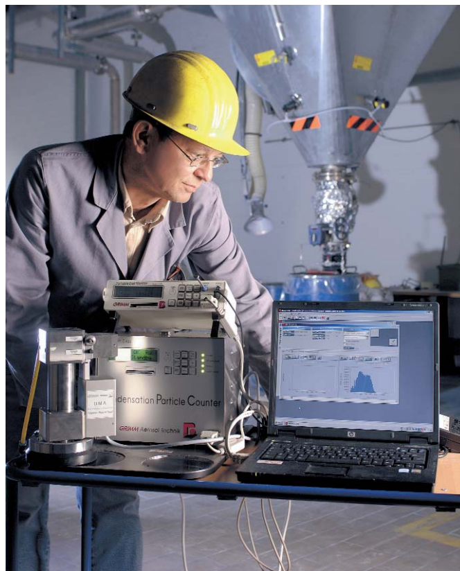
Figure 12: Measuring nanoparticles with a scanning mobility particle sizer (SMPS)
