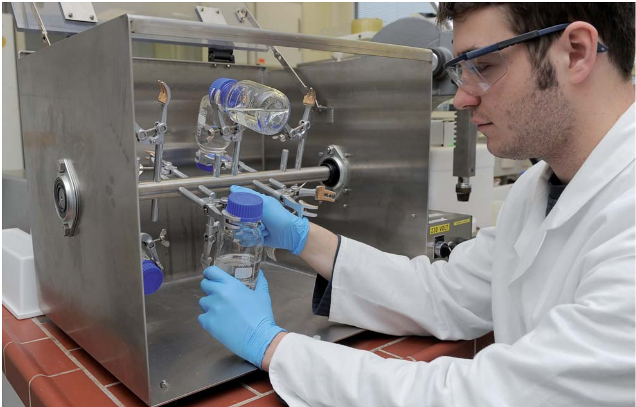
Figure 16: Testing for nanoclay migration from doped plastics
