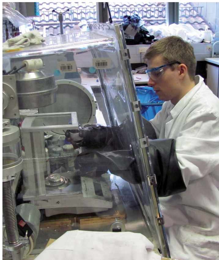
Figure 20: Measuring out fine dusts and nanoparticles in a glove box
