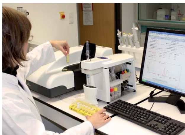
Figure 3: Device for measuring particle size distribution
