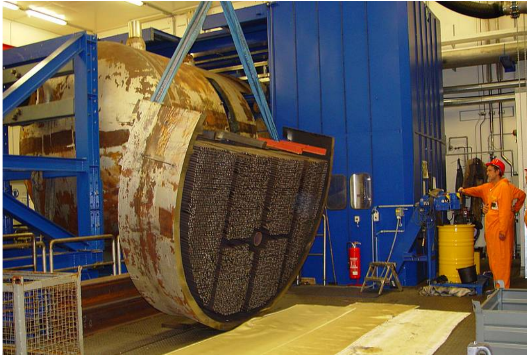
Figure D-16: Segmentation of a steam generator by sawing procedures at ZLN (Copyright: EWN)
