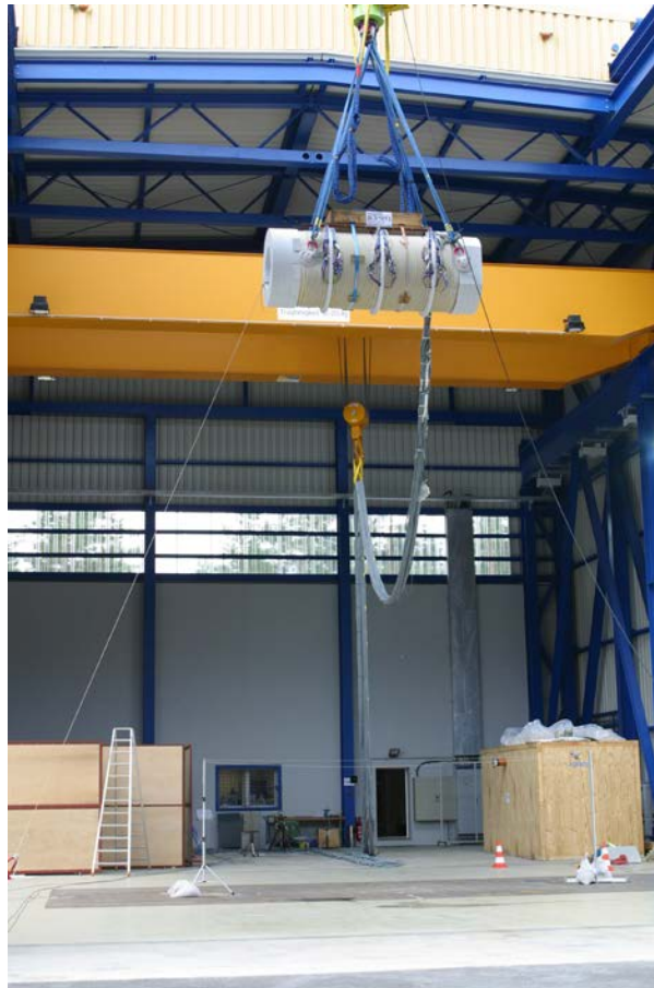
Figure G-1: Drop test of a transport and storage cask (cooled down to -40^{\circ}\text{C} ) for vitrified waste at the test facility of the Federal Institute for Materials Research and Testing (BAM) within the framework of an approval procedure under traffic law (Copyright: BAM)
