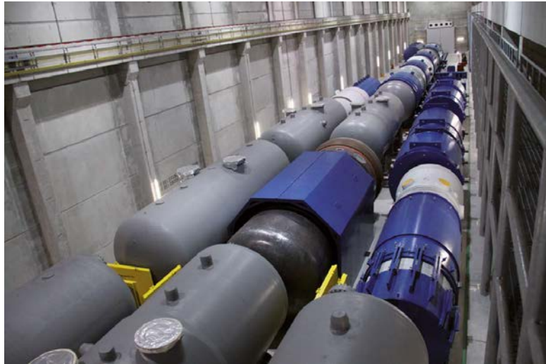
Figure D-9: Decay storage of large components (steam generator, reactor pressure vessel) at the ZLN (Copyright: EWN)
